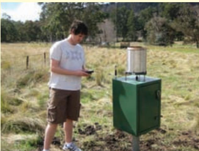
*Testing the radio signal from an automatic rain-gauge at Nundle, near the head of the Peel River.*
